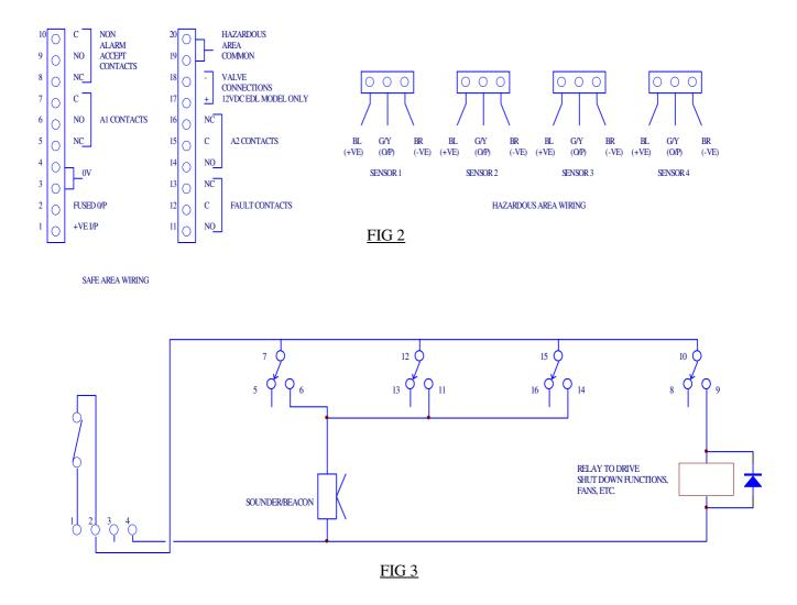
Relay contact rating: 2A at 240VAC Non Inductive
